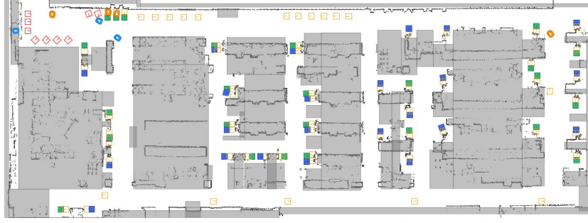
Fig. 2. Factory map with scanned floor plan, nogo-areas (grey), and docking and charging stations
